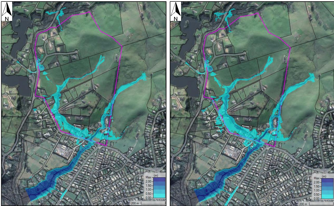
Figure 4-8: Proposed Scenario Model Results – 10% AEP (left) and 1% AEP (right) peak flood depths
