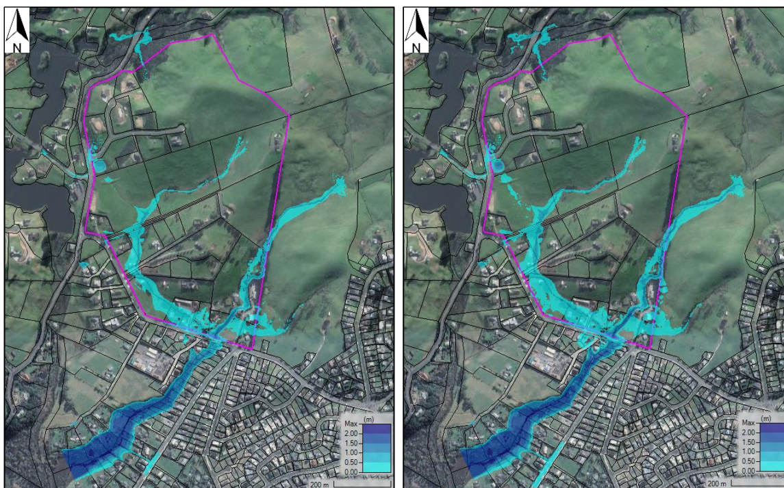
Figure 4-6: Current Scenario Model Results – 10% AEP (left) and 1% AEP (right) peak flood depths.
